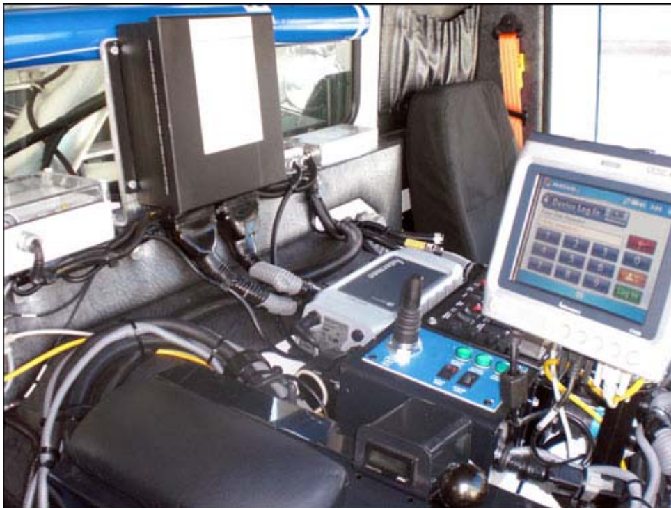
Three trucks were equipped with Intermec CV30 onboard computers, wired to an Intermec IV7 reader.
